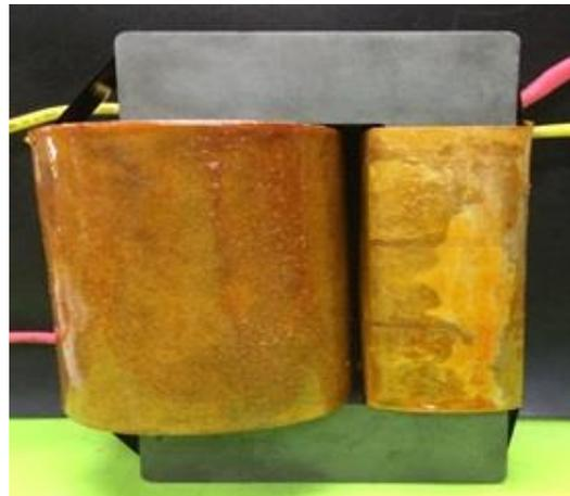
Fig.8. Fly back transformer
