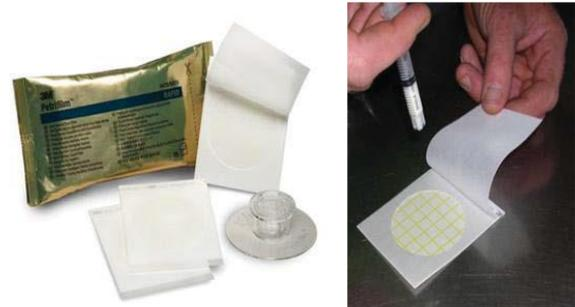
Fig.11. (a) 3M Petrifilm-E.coli Count Plate Sheet and Liquid droplet test.
