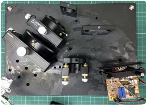
Fig. 2. Implemented spectrometer
