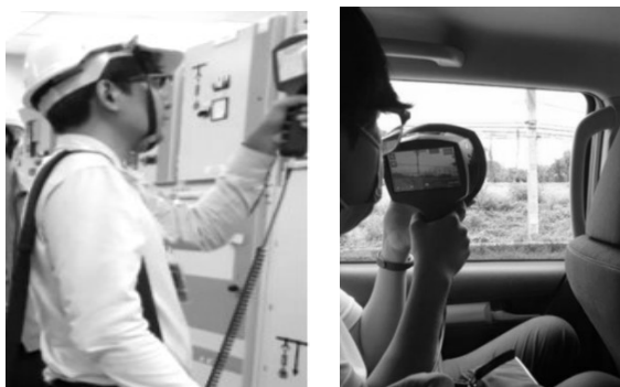
Fig. 3. Mobile acoustic partial discharge detector named NL camera.
