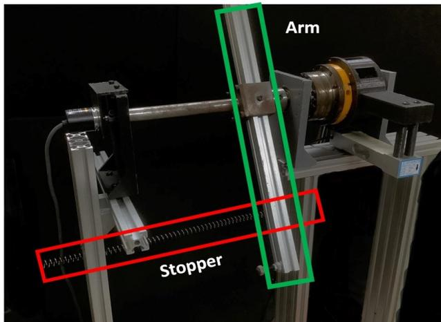
Fig. 9 Simulation of the operate of the robot arm when it collides
