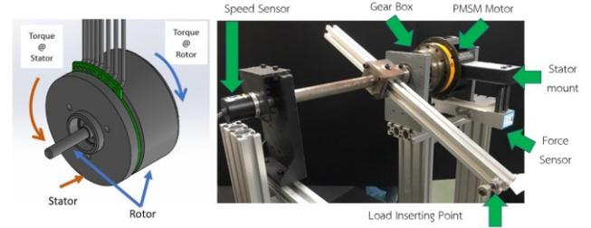
Fig. 3 Torque measurement; Torque of motor (Left) and Low-cost motor test bench (Right)
