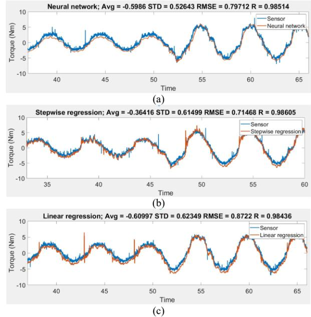
Fig.8 The comparison of torque estimation and error at 1200 rpm (a)The Result of Neural Networks (b) Result of Stepwise regression (c) Result of Linear regression
