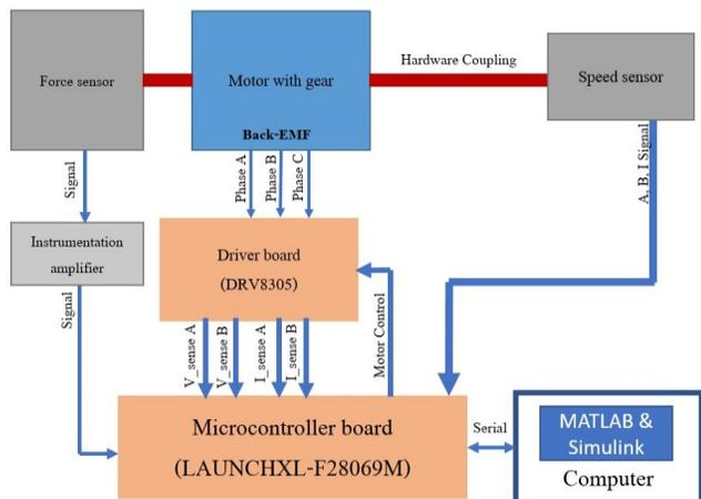
Fig. 4 Schematic diagram of low-cost motor test bench
