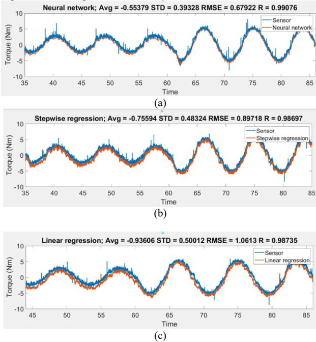
Fig.6 The comparison of torque estimation and error at 700 rpm (a)The Result of Neural Networks (b) Result of Stepwise regression (c) Result of Linear regression
