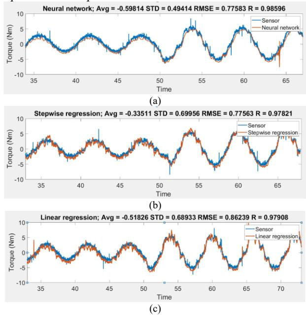
Fig. 7 Fig.7 The comparison of torque estimation and error at 1000 rpm (a) The Result of Neural Networks (b) Result of Stepwise regression (c) Result of Linear regression
