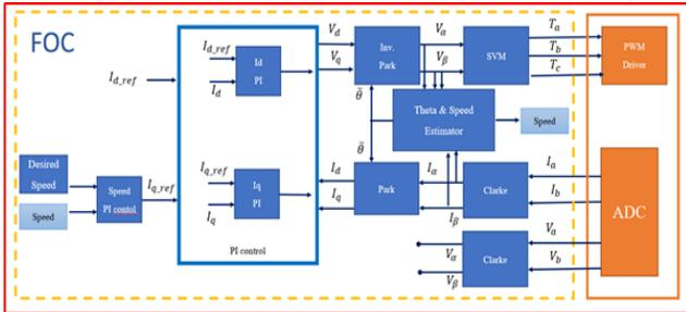
Fig. 1. PMSM control diagram
