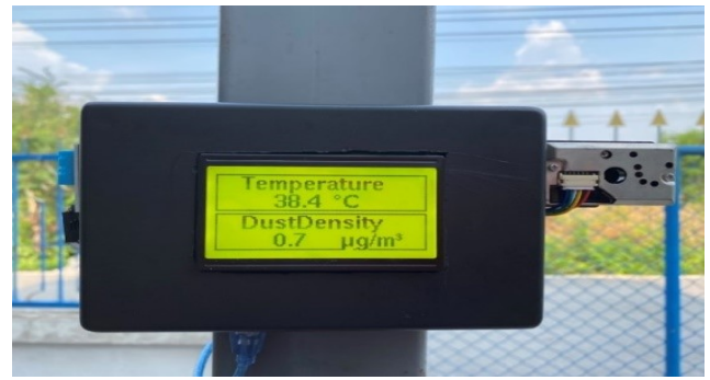
Fig. 22. An example of dust sensor and temperature sensor display
