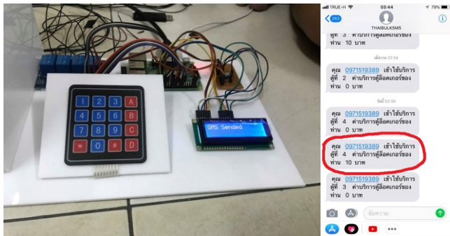
Fig. 25. An example of real testing of SMS sending/receiving process
