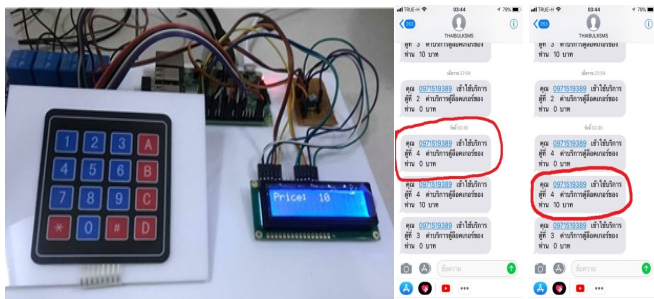
Fig. 12. An example of time metering fee display on user mobile phone after log-off from the smart e- locker engine system
