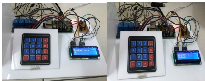
Fig. 14. An example of LK1 is in locked and unlocked status
