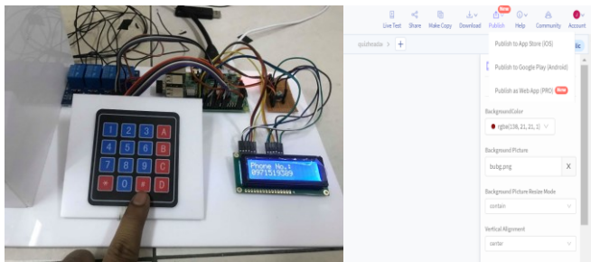
Fig. 11. An example of key pad or mobile phone registration process
