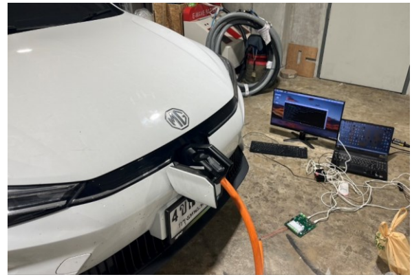
Fig. 8 Testing charging system program with MG ES
