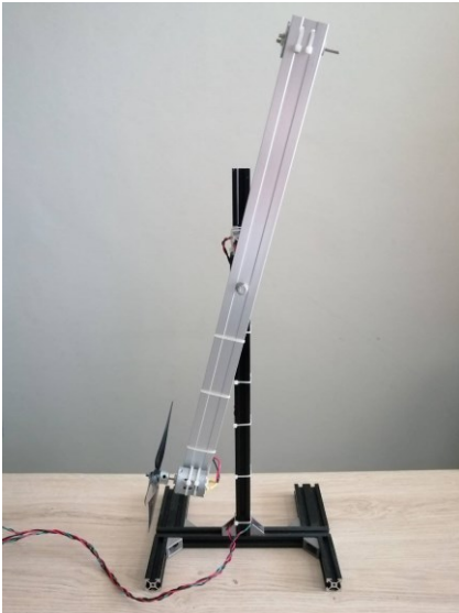
Fig. 2 Experiment kit of aero-pendulum
